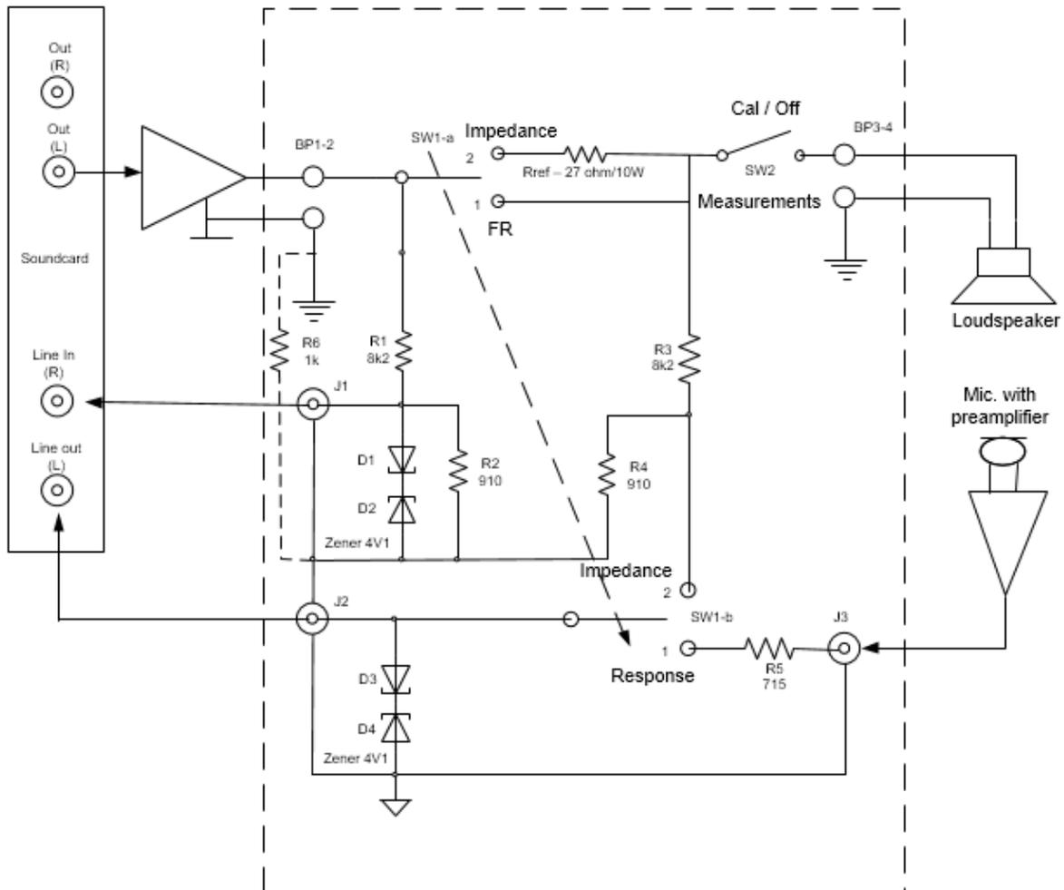
**Note 1** Power amplifier / loudspeaker ground and output low-level grounds are separated by a 1kOhm resistance.
