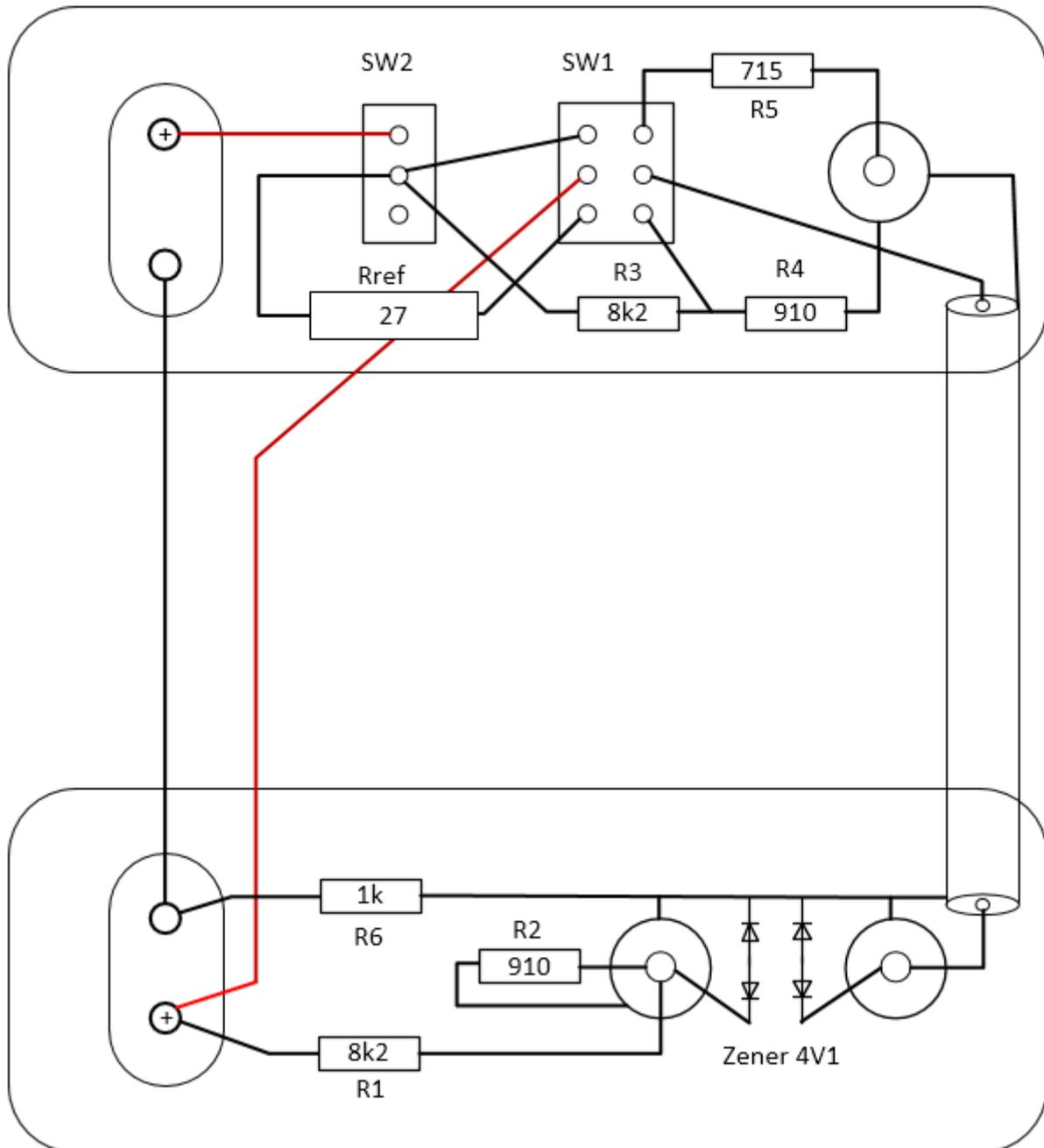
Figure 4. Connection plan for ARTA-Measuring box
