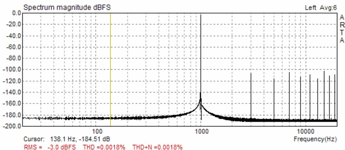
**Figure 2** ARTA 64-bit processed FFT spectrum of a 1 kHz signal - measured with Terratec EWX 24/96 SPIDF I/O (loop-back mode, 16-bit resolution with no dither applied, Kaiser window)
