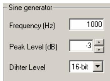
**Figure 4** Adding dither noise to sine generator output
