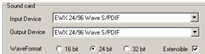
**Figure 7** Soundcard 24-bit resolution setup
