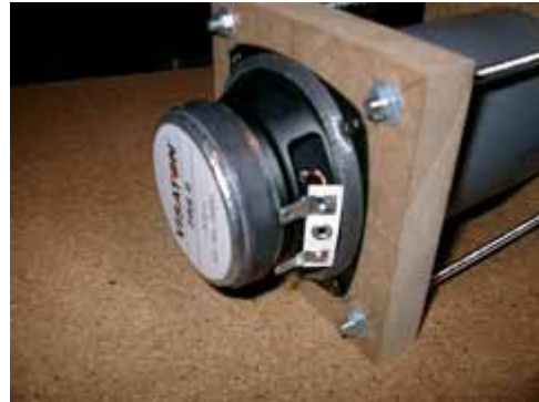
Figure 3.2 Rear view of the completed chamber with driver
