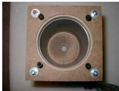
Figure 3.6 Rear panel (driver side), exterior view with nut inserting the driver
