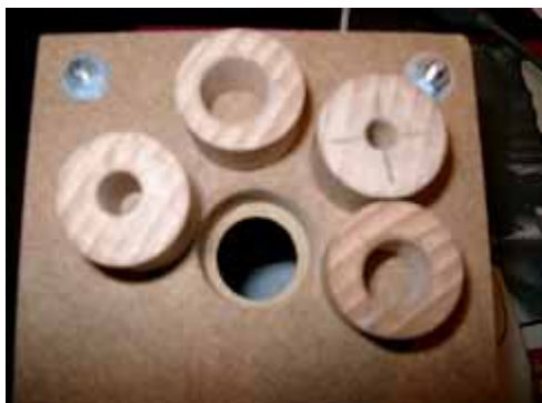
Figure 3.5 Front (microphone) side with hole for 25 mm rod adapter for microphones
