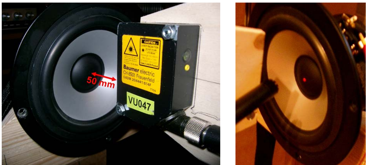
Figure 5: Arrangement of laser and microphone in front of the membrane
