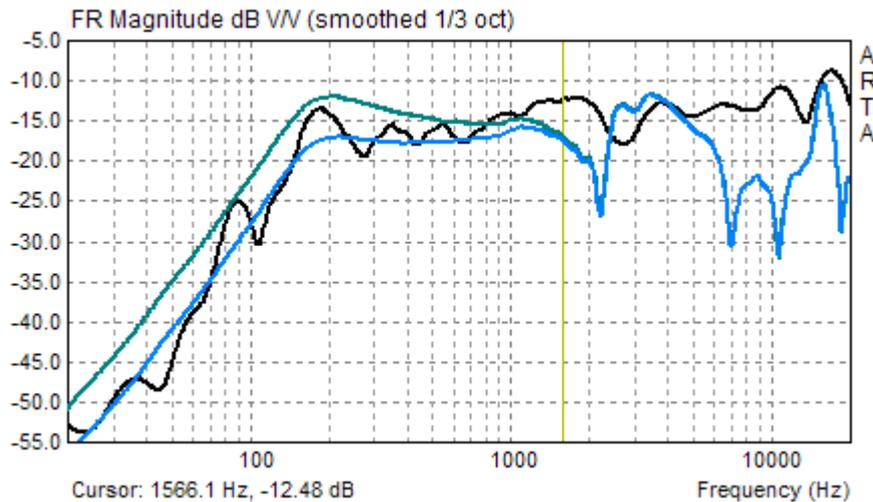
We see that the frequency response measured at 48 cm (black) has high ripple, due to room resonances, but generally it is very close to the estimated free-field response (blue).
