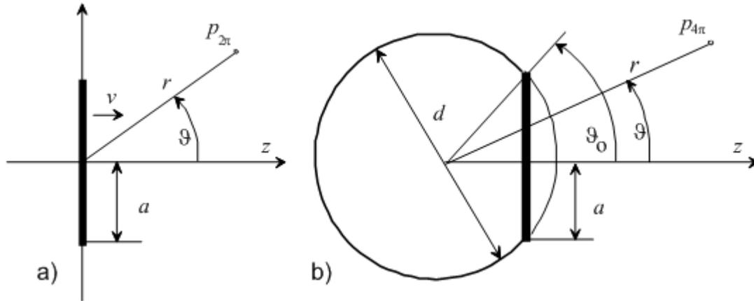
**Figure 5.** a) Loudspeaker with radius  $a$ , mounted on an infinite baffle
