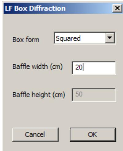
Now we apply LF diffraction correction by the command **Edit->LF box diffraction** and following dialog box.
