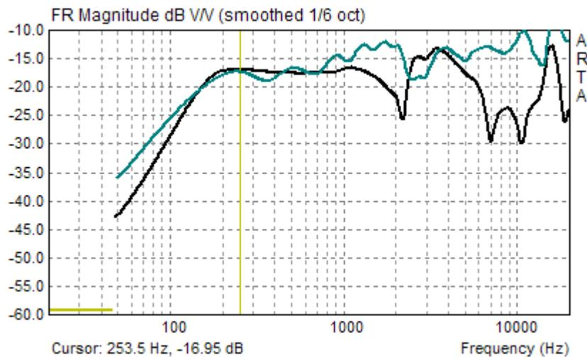
At 235 Hz both responses have same level so we will choose this frequency as a point for joining the two curves. We execute now two commands
