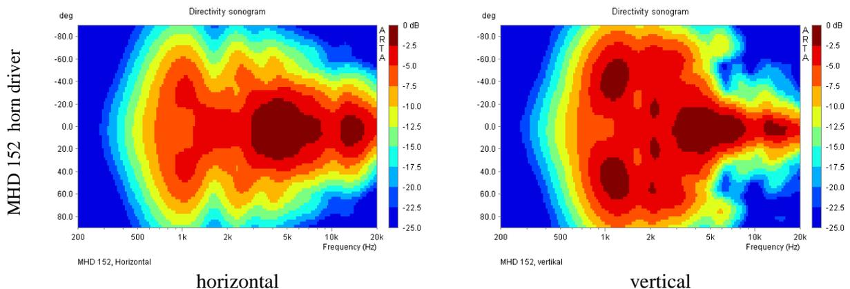
**Figure 12.** high frequency horn, measured horizontally and vertically
