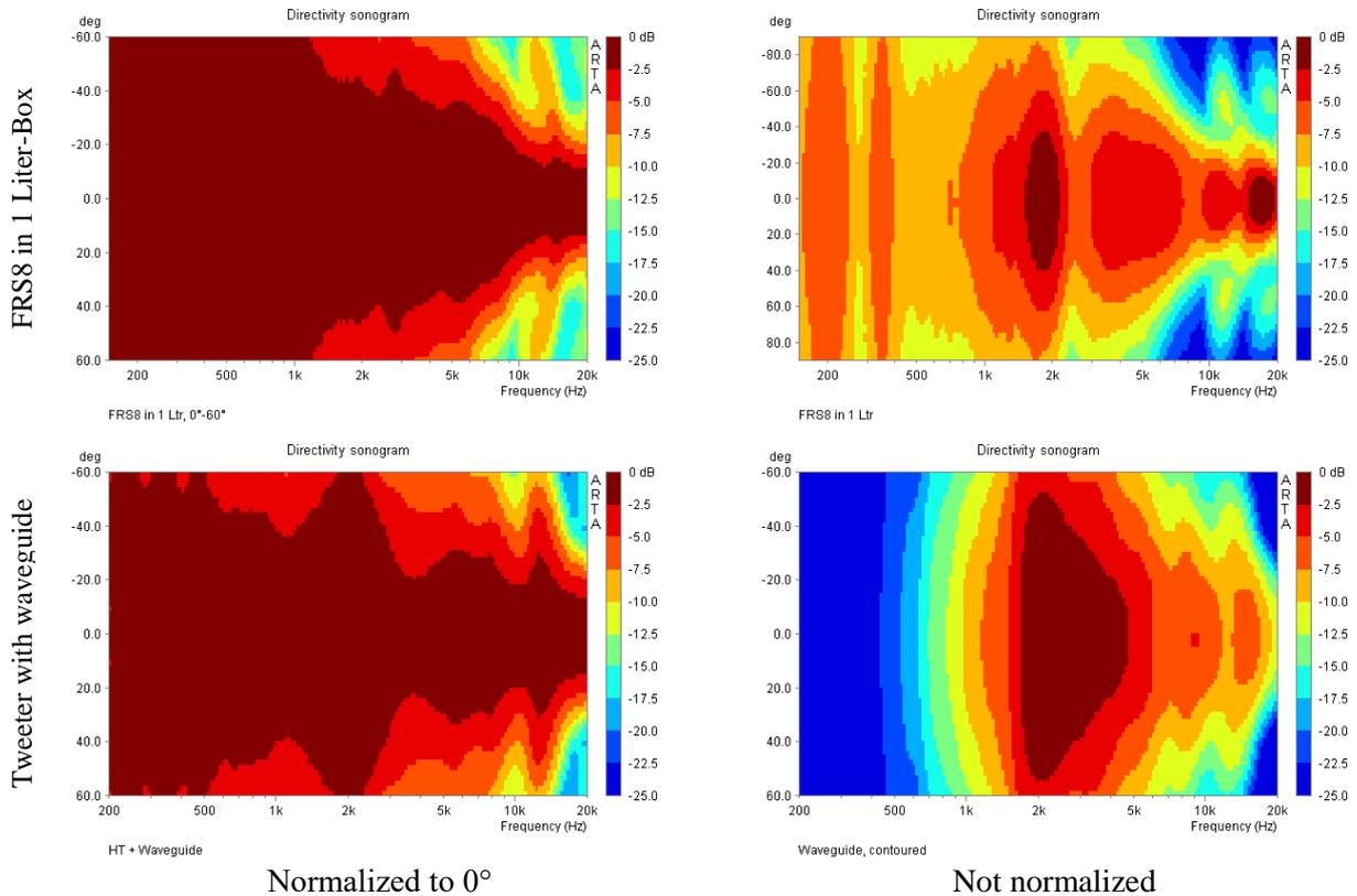
**Figure 11.** Broad-band speaker and tweeter with wave guide
