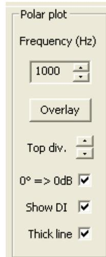
The checkbox "**Show DI**" determines whether and indication for the behavior of the target should be shown. When this is activated, indication of the DI will appear below the polar diagram
