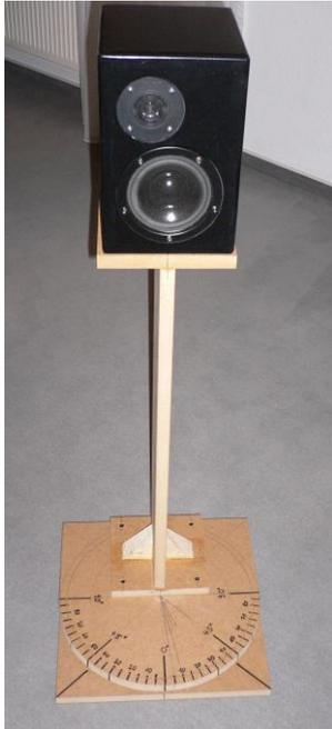
Usually the speaker is measured on a turntable with a scale to show the angle (see Figure 1.). To obtain the full-sphere characteristics, individual frequency responses have to be given for each angle increment.
