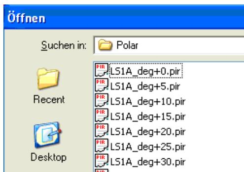
A special feature of the measurement which hasn't yet been explained is that the data is stored using a special nomenclature for the file name. It is composed as follows: Name\_degSignAngle.pir where Sign is '+' or '-', and Angle is given in degrees.
