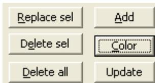
After selecting "**Overlay**", the "**Polar Overlay Manager**" (see Figure 5), with any chosen frequency as an overlay shown separately on or off, deleted or added. With "**Color**" the colors of the curves in the framework of the color palette are modifiable.
