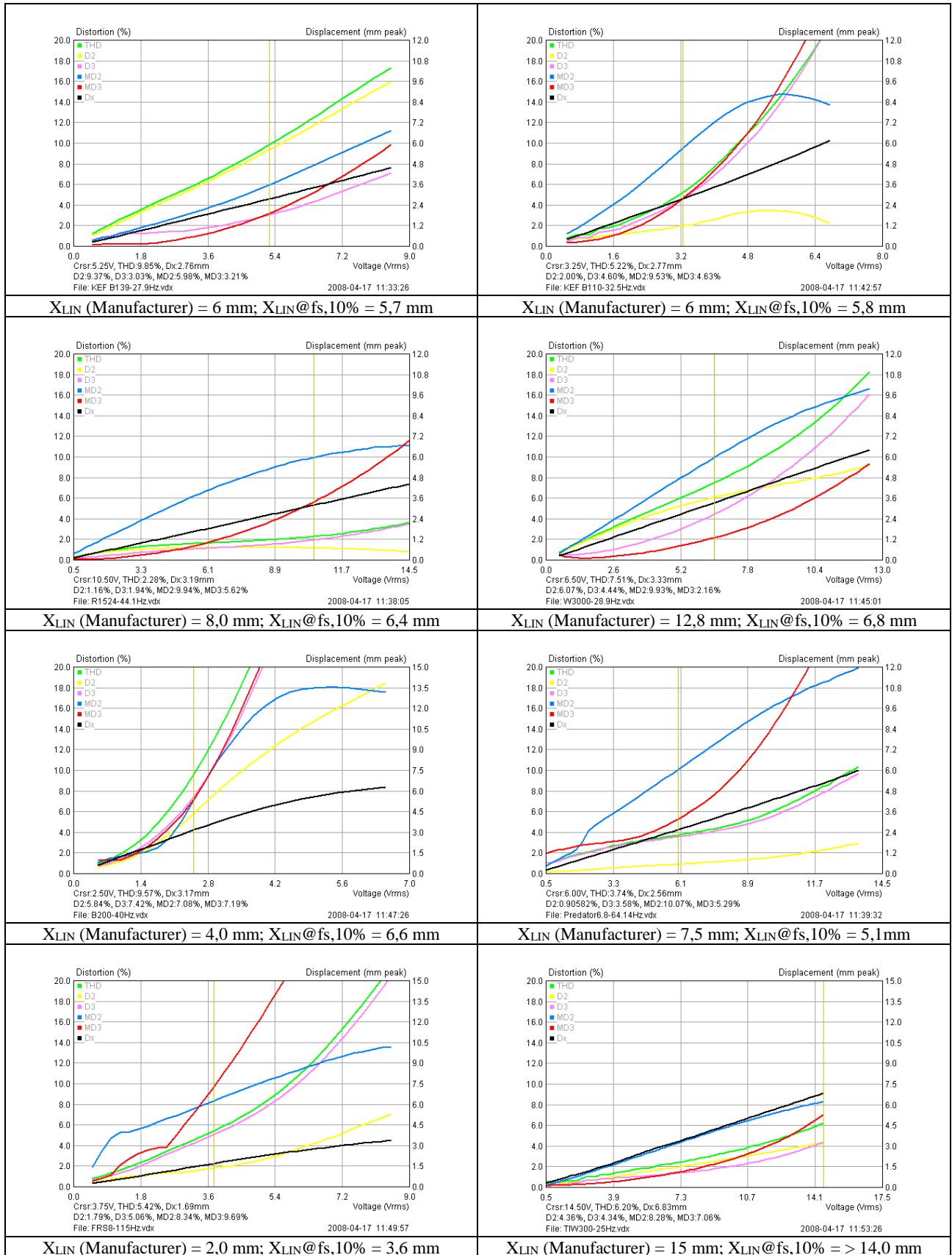
Figure 8. Measured results for a collection of different woofers
