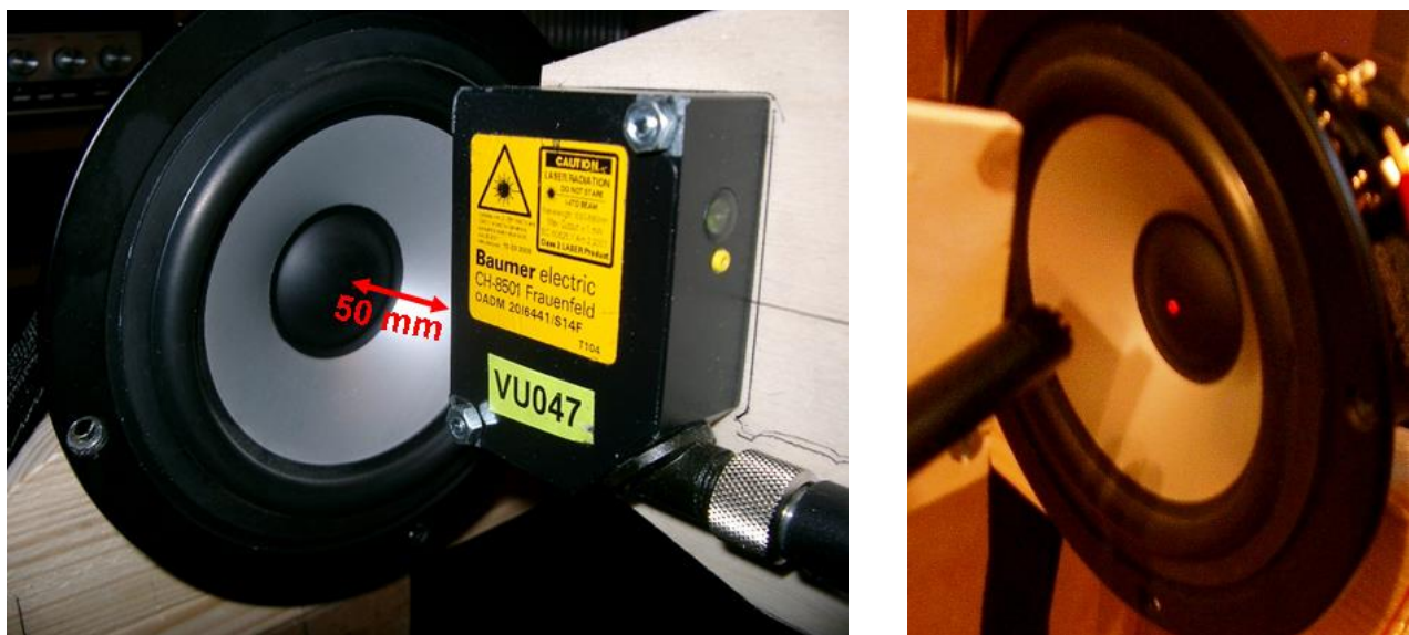
Figure 4: Arrangement of laser and microphone in front of the membrane
